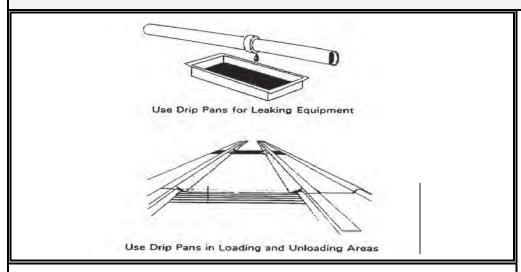
Drip pans are small depressions or pans used to contain very small volumes of leaks, drips, and spills that occur at a facility. Drip pans can be depressions in concrete, asphalt, or other impenetrable material. They can be made of metal, plastic, or any material that does not react with the dripped chemicals. Drip pans can be temporary or permanent.
